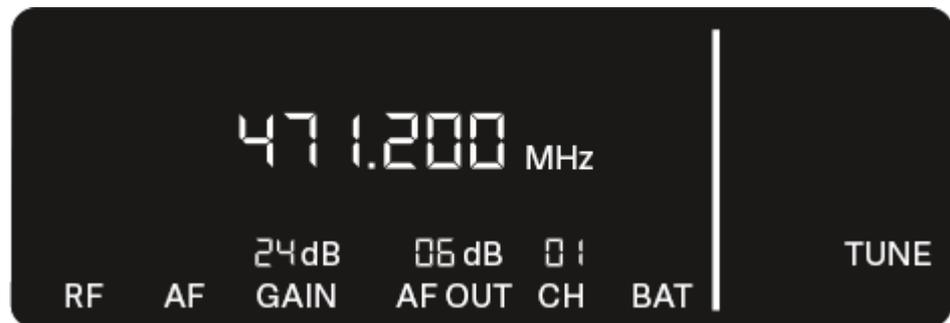
▷ Press the **UP** or **DOWN** buttons to finely adjust the frequency in the kilohertz range.
