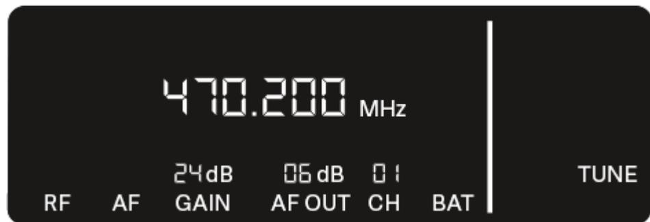
▷ Press the **UP** or **DOWN** button to set the frequency in the megahertz range.
